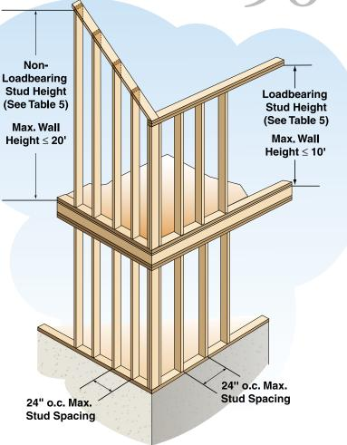
Figure 10. Maximum Wall and Stud Height and Stud Spacing
