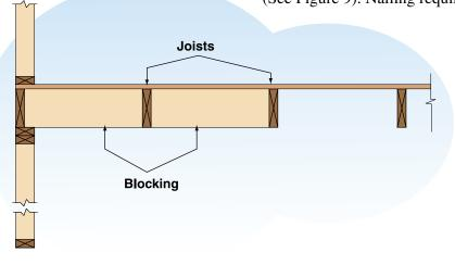
Figure 9. Floor Bracing
