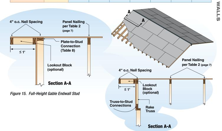
Figure 16. Rake Truss
