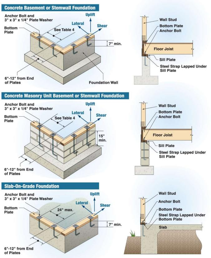
Figure 5. Anchor Bolts Resisting Uplift, Lateral, and Shear Loads.
